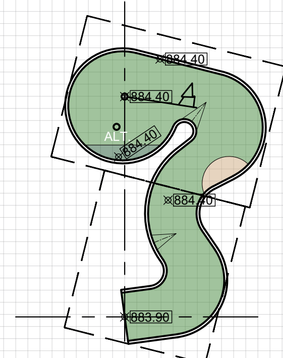
HOLE # 12 - PAR 3 CONCRETE AREA: 210 SQ FT CARPET AREA: 190 SQ FT CARPET LENGTH (12' ROLL): 32 FT EDGING LENGTH: 90 FT
