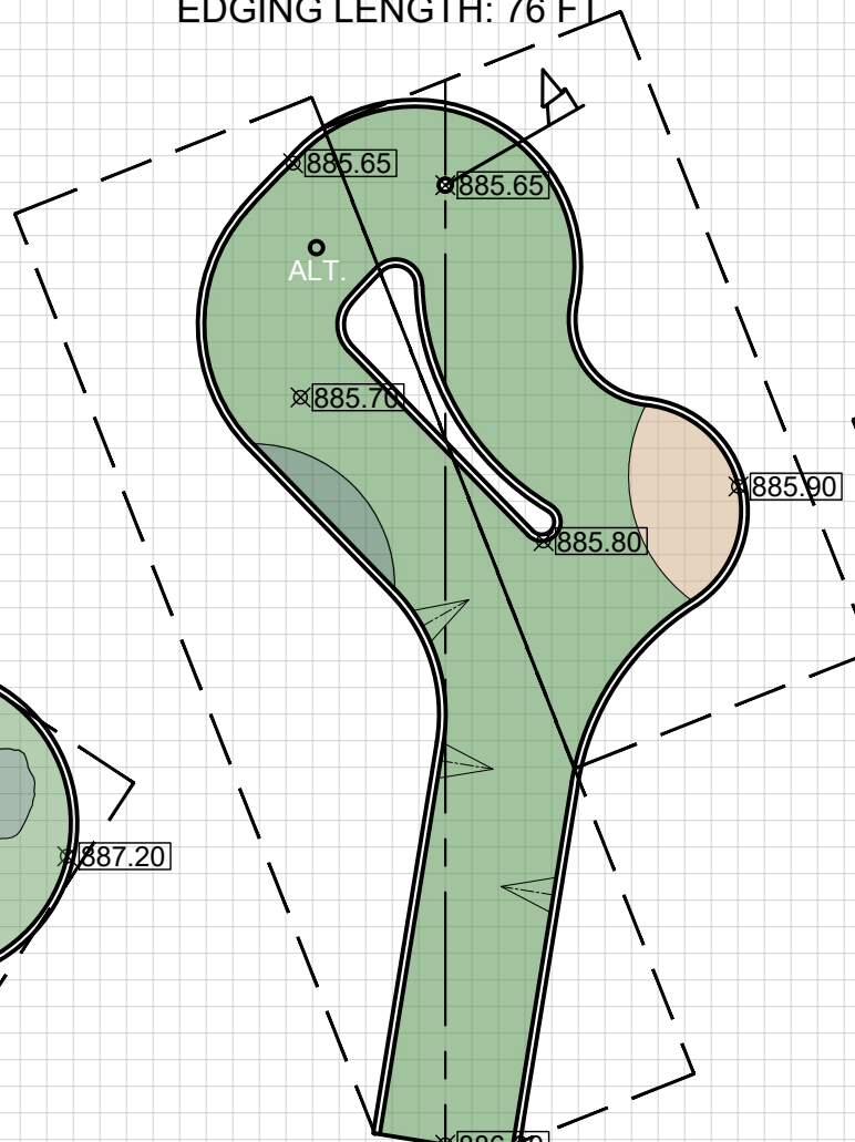
HOLE # 10 - PAR 3 CONCRETE AREA: 370 SQ FT CARPET AREA: 339 SQ FT CARPET LENGTH (12' ROLL): 62 FT EDGING LENGTH: 124 FT
